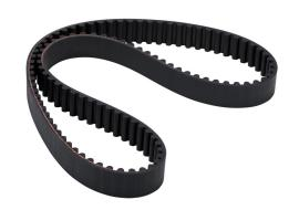
SureMotion timing belt, 8mm 8M pitch, 20mm wide, 105 tooth, 840mm pitch length (circumference), neoprene, fiberglass reinforced.
