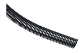
Murrplastik EW-PAB solid flexible corrugated tubing, modified polyamide 6, M40/P36 tubing size, black, 82ft/25m coil length.
