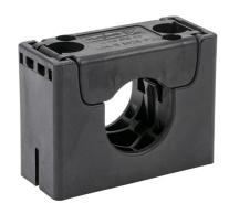
Murrplastik UH-S clamp, M25/P21 tubing size, black. Package of 5. For use with EW-PAB and EW-PRF series flexible corrugated solid tubing and EWT-PA series flexible corrugated split tubing.
