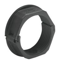
Murrplastik connector, split lock nut, M25 x 1.5mm thread type, black. Package of 5. For use with part number 836016 and 836018 SVT threaded straight connectors.
