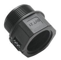
Murrplastik SVT connector, threaded straight, M32x1.5/P21 trade size, M32 x 1.5mm thread type, black. Package of 5. For use with EWT-PA series two-piece split conduit.
