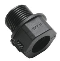
Murrplastik SVT connector, threaded straight, M20x1.5/P11 trade size, M20 x 1.5mm thread type, black. Package of 5. For use with EWT-PA series two-piece split conduit.
