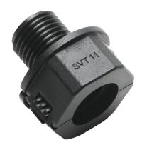
Murrplastik SVT connector, threaded straight, M16x1.5/P11 trade size, M16 x 1.5mm thread type, black. Package of 5. For use with EWT-PA series two-piece split conduit.
