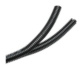
Murrplastik EWT-PA two-piece split flexible electrical conduit, polyamide, M20/P16 trade size, black, 32.8ft/10m coil length.
