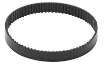
SureMotion timing belt, 0.08in MXL pitch, 1/4in wide, 82 tooth, 6.6in pitch length (circumference), polyurethane, polyester reinforced. Package of 3.
