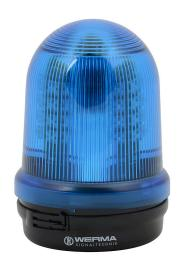
WERMA LED industrial signal beacon, 98mm, blue, permanent/blinking/rotating (1.66 Hz ON for 298ms, 180rpm), IP65, base mount, 24 VDC.
