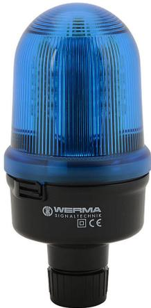
WERMA LED industrial signal beacon, 98mm, blue, permanent or blinking (1.5 Hz ON for 350ms), IP65, tube mount, 24 VDC.
