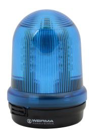
WERMA LED industrial signal beacon, 98mm, blue, permanent or blinking (1.5 Hz ON for 350ms), IP65, base mount, 24 VDC.
