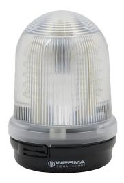
WERMA LED industrial signal beacon, 98mm, clear/white, EVS (Enhanced Visibility System) flashing (random flashing), IP65, base mount, 115-230 VAC.
