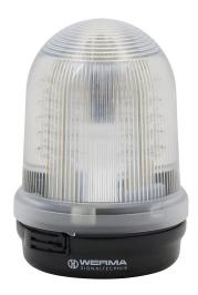
WERMA LED industrial signal beacon, 98mm, clear/white, double flash, IP65, base mount, 115-230 VAC.
