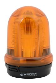
WERMA LED industrial signal beacon, 98mm, yellow, rotating (180rpm), IP65, base mount, 24 VDC.
