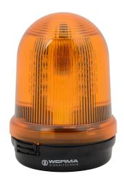
WERMA LED industrial signal beacon, 98mm, yellow, permanent or blinking (1.5 Hz ON for 350ms), IP65, base mount, 24 VDC.
