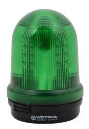
WERMA LED industrial signal beacon, 98mm, green, permanent/blinking/rotating (1.66 Hz ON for 298ms, 180rpm), IP65, base mount, 24 VDC.
