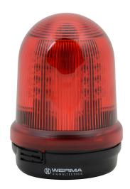
WERMA LED industrial signal beacon, 98mm, red, permanent/blinking/rotating (1.66 Hz ON for 298ms, 180rpm), IP65, base mount, 24 VDC.
