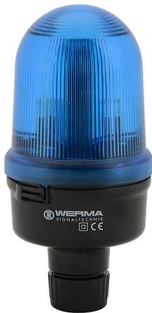
WERMA Xenon tube industrial signal beacon, 98mm, blue, flashing strobe (1 Hz flash frequency), IP65, tube mount, 24 VDC.
