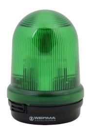
WERMA Xenon tube industrial signal beacon, 98mm, green, flashing strobe (1 Hz flash frequency), IP65, base mount, 24 VDC.
