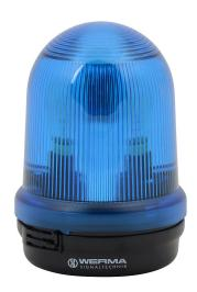
WERMA incandescent industrial signal beacon, 98mm, blue, blinking (1.84 Hz ON for 284ms), IP65, base mount, 115 VAC.
