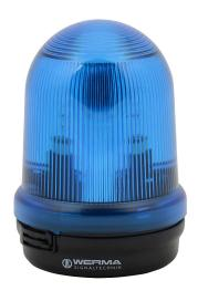
WERMA incandescent industrial signal beacon, 98mm, blue, blinking (1.84 Hz ON for 284ms), IP65, base mount, 24 VAC/VDC.
