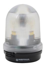
WERMA incandescent industrial signal beacon, 98mm, clear/white, blinking (1.84 Hz ON for 284ms), IP65, base mount, 115 VAC.
