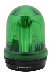
WERMA incandescent industrial signal beacon, 98mm, green, blinking (1.84 Hz ON for 284ms), IP65, base mount, 115 VAC.
