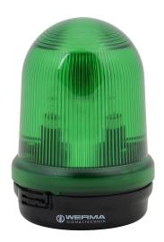
WERMA incandescent industrial signal beacon, 98mm, green, blinking (1.84 Hz ON for 284ms), IP65, base mount, 24 VAC/VDC.
