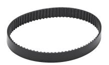
SureMotion timing belt, 0.08in MXL pitch, 1/4in wide, 81 tooth, 6.5in pitch length (circumference), polyurethane, polyester reinforced. Package of 3.
