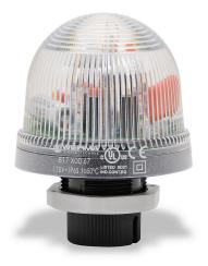
WERMA Xenon tube industrial signal beacon, 75mm, clear/white, flashing strobe (1 Hz flash frequency), IP65, 37mm (PG 29) mount, 115 VAC.
