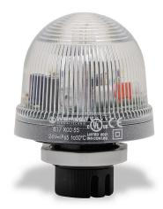
WERMA Xenon tube industrial signal beacon, 75mm, clear/white, flashing strobe (1 Hz flash frequency), IP65, 37mm (PG 29) mount, 24 VDC.
