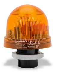
WERMA Xenon tube industrial signal beacon, 75mm, yellow, flashing strobe (1 Hz flash frequency), IP65, 37mm (PG 29) mount, 115 VAC.
