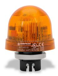
WERMA Xenon tube industrial signal beacon, 75mm, yellow, flashing strobe (1 Hz flash frequency), IP65, 37mm (PG 29) mount, 24 VDC.
