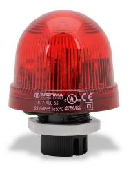
WERMA Xenon tube industrial signal beacon, 75mm, red, flashing strobe (1 Hz flash frequency), IP65, 37mm (PG 29) mount, 24 VDC.
