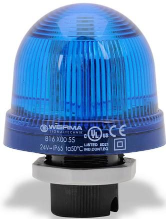
WERMA LED industrial signal beacon, 75mm, blue, permanent, IP65, 37mm (PG 29) mount, 24 VAC/VDC.
