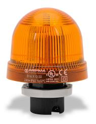
WERMA LED industrial signal beacon, 75mm, yellow, blinking (1 Hz ON for 530ms), IP65, 37mm (PG 29) mount, 24 VAC/VDC.
