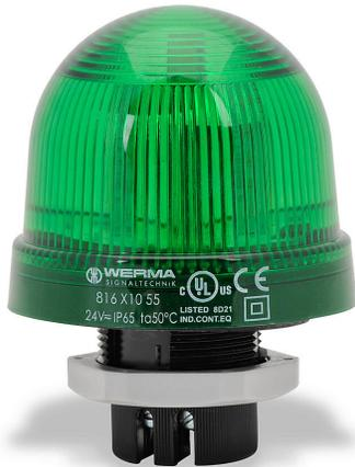
WERMA LED industrial signal beacon, 75mm, green, blinking (1 Hz ON for 530ms), IP65, 37mm (PG 29) mount, 24 VAC/VDC.
