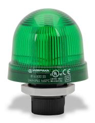
WERMA LED industrial signal beacon, 75mm, green, permanent, IP65, 37mm (PG 29) mount, 24 VAC/VDC.
