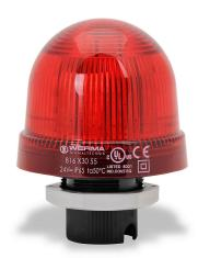
WERMA LED industrial signal beacon, 75mm, red, rotating (120rpm), IP65, 37mm (PG 29) mount, 24 VAC/VDC.
