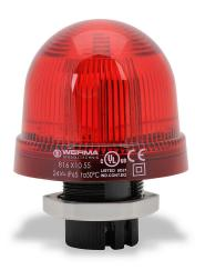
WERMA LED industrial signal beacon, 75mm, red, blinking (1 Hz ON for 530ms), IP65, 37mm (PG 29) mount, 24 VAC/VDC.
