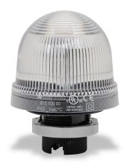
WERMA incandescent industrial signal beacon, 75mm, clear/white, permanent, IP65, 37mm (PG 29) mount, 12-240 VAC/VDC. Requires incandescent bulb.
