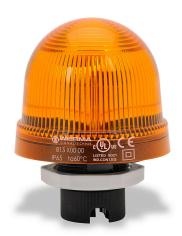
WERMA incandescent industrial signal beacon, 75mm, yellow, permanent, IP65, 37mm (PG 29) mount, 12-240 VAC/VDC. Requires incandescent bulb.
