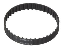
SureMotion timing belt, 1/5in XL pitch, 3/8in wide, 40 tooth, 8in pitch length (circumference), neoprene, fiberglass reinforced.
