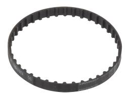
SureMotion timing belt, 1/5in XL pitch, 1/4in wide, 40 tooth, 8in pitch length (circumference), neoprene, fiberglass reinforced.
