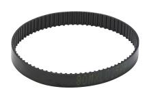
SureMotion timing belt, 0.08in MXL pitch, 1/4in wide, 80 tooth, 6.4in pitch length (circumference), polyurethane, polyester reinforced. Package of 3.
