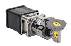
IDEM Skorpion series solenoid control switch, rotary key, A105 coded, (4) N.C./(2) N.O. contact(s), die-cast aluminum alloy. For use with A105 coded Skorpion trapped key interlock systems. (1) M-CS-SKR solenoid control switch and (1) SK-KEY key included.
