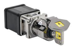
IDEM Skorpion series solenoid control switch, rotary key, A104 coded, (4) N.C./(2) N.O. contact(s), die-cast aluminum alloy. For use with A104 coded Skorpion trapped key interlock systems. (1) M-CS-SKR solenoid control switch and (1) SK-KEY key included.
