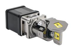
IDEM Skorpion series solenoid control switch, rotary key, A103 coded, (4) N.C./(2) N.O. contact(s), die-cast aluminum alloy. For use with A103 coded Skorpion trapped key interlock systems. (1) M-CS-SKR solenoid control switch and (1) SK-KEY key included.
