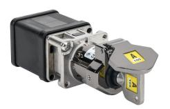
IDEM Skorpion series control switch, rotary key, A105 coded, (4) N.C./(2) N.O. contact(s), die-cast aluminum alloy. For use with A105 coded Skorpion trapped key interlock systems. (1) M-CS control switch and (1) SK-KEY key included.
