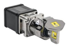
IDEM Skorpion series control switch, rotary key, A104 coded, (4) N.C./(2) N.O. contact(s), die-cast aluminum alloy. For use with A104 coded Skorpion trapped key interlock systems. (1) M-CS control switch and (1) SK-KEY key included.
