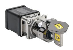
IDEM Skorpion series control switch, rotary key, A102 coded, (4) N.C./(2) N.O. contact(s), die-cast aluminum alloy. For use with A102 coded Skorpion trapped key interlock systems. (1) M-CS control switch and (1) SK-KEY key included.
