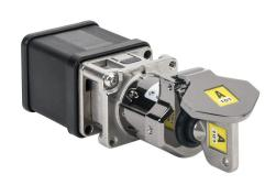
IDEM Skorpion series control switch, rotary key, A101 coded, (4) N.C./(2) N.O. contact(s), die-cast aluminum alloy. For use with A101 coded Skorpion trapped key interlock systems. (1) M-CS control switch and (1) SK-KEY key included.
