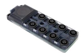
Exact 12 passive distribution block, 8 ports, 5-pin M12 sockets, 5-wire, 24 VDC, 4A, power and PNP LED indicator(s), panel mount plug in, IP67. Terminal blocks and marking tags included.
